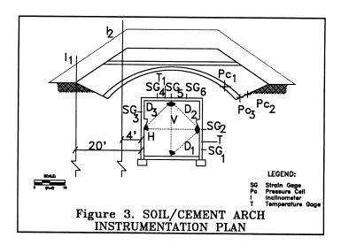
Construction Procedures. The construction of the soil/cement arch involved excavation of 3 feet of the existing soils from elevation 98 to 95 over the top of the tunnel. Soil was then loosely backfilled over the tunnel in the configuration of the arch (soil type 2 shown on Figure 2). The haunches for the support of the arch were excavated above the sides of the tunnel.
