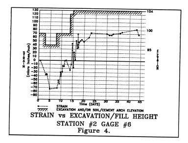
The change in strain and correlated change in stress based on the relationship established during the removal of the overburden soil, appears to indicate that the tunnel sidewalls are relatively flexible and that an active earth pressure condition exists. For this case, the finite element analysis predicted an increase in stress of 10% to 20%. The measured change was 6% to 20%.
